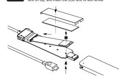
4 Push back the PCB tray and lock with the screws
