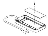
4 Cover the top cover and lock the screws. The installation is complete.
