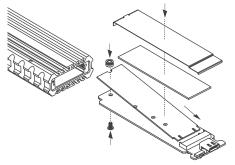
Push back the PCB tray and lock with the screws, and insert the pull ring assembly. The installation is complete.
