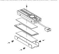
3 Insert the M.2 card heat sink into the plug M key connector of the M Key computer motherboard and lock the screw.
