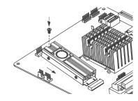
Then insert the 4 PIN plug into the 4 PIN socket on the motherboard of the computer and the installation is complete.
