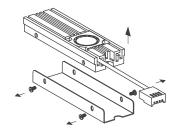
2 Install thermal silicon, M.2 SSD card, heat sink, and lock 4 screws.
